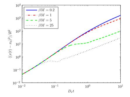
FIG. 10: Mean square displacement of a spherical particle with additional constant external torque for  $\beta RF_0 = 10$ ,  $\phi_0 = 0$  and different values of  $\beta M$ .
