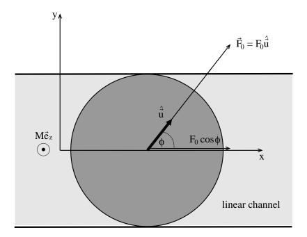
FIG. 1: Sketch of the model system: A spherical colloidal particle (dark grey) is confined to a linear channel (light grey) along the x-direction. The self-propulsion is modelled by a constant effective force  $\vec{F_0}$  along the particle orientation  $\hat{\vec{u}}$ . The latter is constrained to rotate in the xy-plane. Only the projected force  $F_0 \cos \phi$  drives the particle along the channel. A systematic, time-dependent torque  $\vec{M}(t) = M(t)\hat{\vec{e}}_z$  is also indicated.
