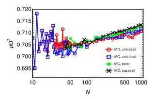
FIG. 4. Maximum obtained surface density  $\rho$  as a function of the cluster size N for aspect ratio L/D=0.5. The lines indicate different optimization methods as indicated, with points specifying all investigated choices of N.
