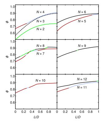
FIG. 3. Maximum obtained area packing fraction  $\phi$  for small clusters as a function of the aspect ratio L/D for different cluster sizes as indicated. Different colors along the same line indicate different structures as indicated in Tables I and II.
