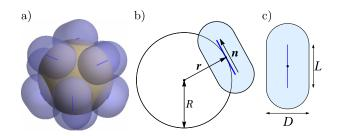
FIG. 2. (a) Depiction of a configuration of 9 rods (L/D=0.5) tangential to a central sphere. (b) Two-dimensional schematic of the model. Shown are the central sphere with radius R, the particles at position  $\mathbf{r}$ , and its orientation vector  $\mathbf{n}$ . (c) Length scales associated with a single rod: the cylinder length L and the rod diameter D.
