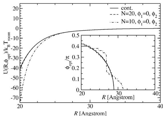
FIGURE 4 Yukawa-segment pair potential per length  $L_p$  as a function of the interaxial separation  $R$  of two DNA molecules, at the optimal angle  $\phi_{2,opt}(R)$ , depicted for  $N = 10, N = 20$  charges as well as for continuous line charges. The dependence of the optimal angle on the interaxial separation  $R$  is shown in the inset.
