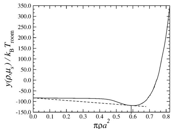
FIGURE 18 Semigrand potential per unit volume  $y(\rho, \mu_s)$  on a line of constant DNA chemical potential for the KL model as a function of the reduced DNA density and for parameters  $\theta = 0.9, f_1 = 0.3, f_2 = 0.7$ , and  $f_3 = 0$ . Also shown (dashed line) is the common tangent connecting the coexisting phase points.
