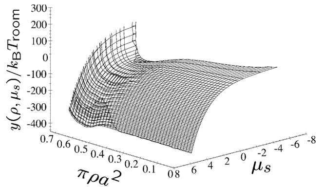
FIGURE 17 Semigrand potential per unit volume  $y(\rho, \mu_s)$  as a function of reduced DNA density and salt chemical potential, for the KL model and parameters  $\theta = 0.9, f_1 = 0.3, f_2 = 0.7$ , and  $f_3 = 0$ .
