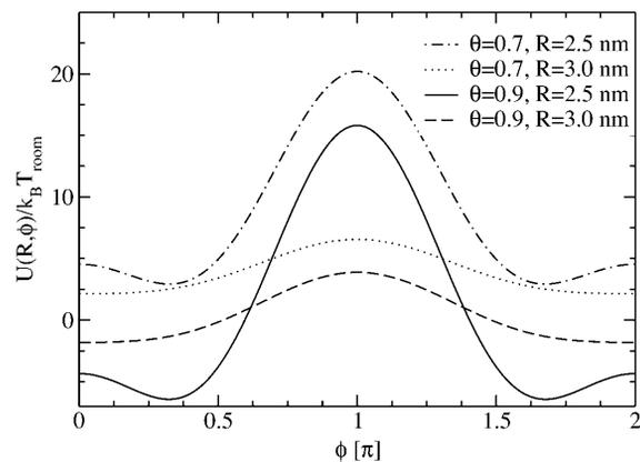
FIGURE 7 Yukawa-segment pair potential for two segments of length  $L_p$  as a function of the mutual azimuthal orientation angle  $\phi$  of two DNA molecules, at fixed interaxial separations as indicated in the legend, for  $\theta = 0.9$  and  $\theta = 0.7$ .  $f_1 = 0.3, f_2 = 0.7$ , and  $f_3 = 0$  were used for the fractions of condensed counterions in the minor and major groove and on the strands, at different interaxial separations, as indicated in the legend.
