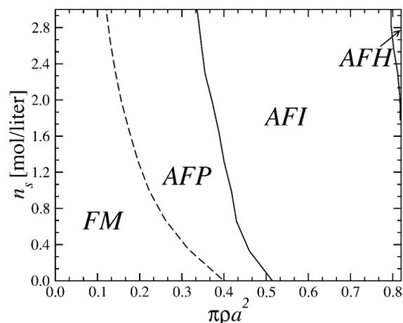
FIGURE 13 Phase diagram of DNA-salt mixtures for the *YS* model as a function of the DNA packing fraction  $\pi\rho a^2$  and salt concentration  $n_s$  in the aggregate:  $\theta = 0.9$ ,  $f_1 = f_2 = 0$ , and  $f_3 = 1$ ; the lattice here is *HEX*. Dashed lines denote second-order magnetic transitions, solid lines first-order ones.
