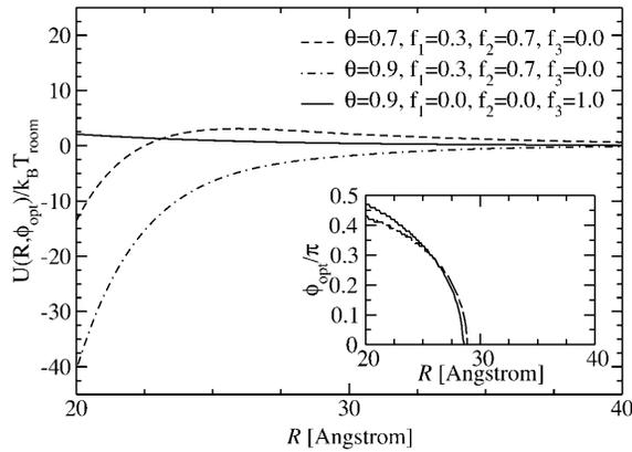
FIGURE 8 Yukawa-segment pair potential for two segments of length  $L_p$  as a function of the interaxial separation  $R$  of two DNA molecules, at the optimal angle  $\phi_{\text{opt}}(R)$ , depicted for different values of the counterion condensation parameter and for different counterion adsorption patterns. The dependence of the optimal angle on the interaxial separation  $R$  is shown in the inset.
