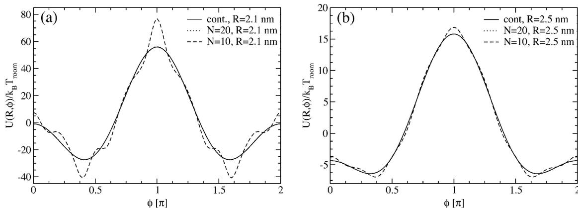
FIGURE 3 Yukawa-segment pair potential per length  $L_p$  as a function of the azimuthal orientation angle  $\phi_2$  with  $\phi_1 = 0$  fixed, at interaxial separations (a)  $R = 2.1$  nm and (b)  $R = 2.5$  nm, for  $\theta = 0.9$  and  $f_1 = 0.3, f_2 = 0.7$ , and  $f_3 = 0$ . At both interaxial separations the potential is displayed for  $N = 10, N = 20$  charges as well as for continuous line charges.
