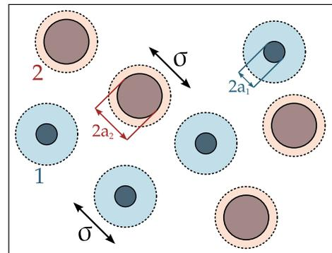
**Figure 4.** Sketch of the mobility-binary system. Two particle species 1 and 2 with the same interaction diameter  $\sigma$  but with different hydrodynamic radii  $a_1$  and  $a_2$  are shown. .
