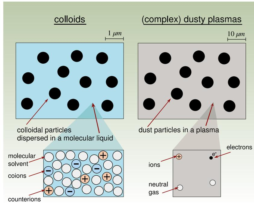
**Figure 1.** Schematic view of colloidal dispersions and complex plasmas: colloidal particles (black spheres in the left picture) are embedded in a molecular liquid containing also microions (counter- and co-ions) while dust particles (black spheres in the right picture) are embedded in a dilute weakly ionized gas.
