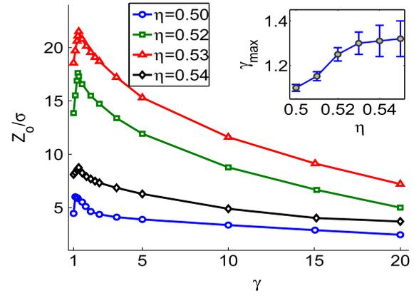
**Figure 8.** Simulation results for the crystal–liquid front position  $z_0$  for different bulk packing fractions  $\eta$  at  $t = 50\tau_3$  as a function of the mobility ratio  $\gamma = D_1/D_2$ . The inset shows the dependence of the value  $\gamma_{\max}$  at which  $z_0$  is maximal on the bulk packing fraction  $\eta$ . The error bars are no larger than the symbol size used.
