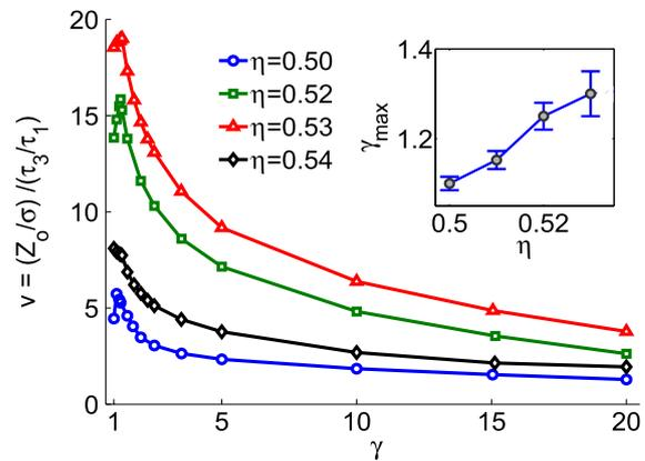
**Figure 9.** Simulation results for the crystal–fluid front velocity  $v$  for different bulk packing fractions at  $t = 50\tau_3$  as a function of the mobility ratio  $\gamma = D_1/D_2$ . The parameter  $\gamma_{\max}$ , which corresponds to the values of  $\gamma$  at which the front velocity reaches a maximum value is shown in the inset. The error bars of calculated velocities do not exceed the size of the symbols used.
