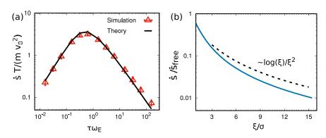
**FIG. 3.** Total entropy production rate. (a) Rescaled entropy production rate  $\dot{s}$   $T/(mv_0^2)$  as a function of  $\tau\omega_E$ . (b) Entropy production rate  $\dot{s}/\dot{s}_{\text{free}}$  as a function of  $\xi/d_0$ . Solid lines are obtained by theoretical predictions, while points are obtained by numerical simulations. The black dashed line is a guide for the eyes for the scaling  $\sim \log(\xi)/\xi^2$ . The parameters are  $N=10^4$  and  $\phi=1.1$ .
