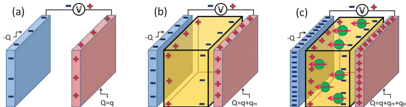
Fig. 1 Schematic illustration of the electrostatic energy storage in capacitors connected to a battery with a voltage  $V$ . Case (a) a capacitor without a dielectric film will be charged up to a charge  $q$ . Case (b) a capacitor with a dielectric film will be charged up to a charge  $q + q_m$ . Case (c) a capacitor with a dielectric film impregnated with high- $k$  inclusions will be charged up to a charge  $q + q_m + q_p$ . For more details, see text.
